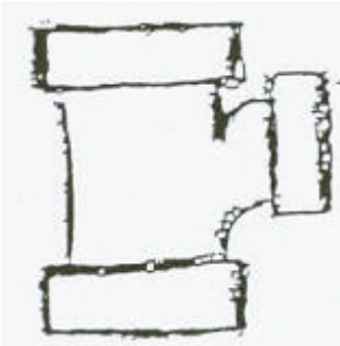
"Tee" may be used in VERTICAL position only
